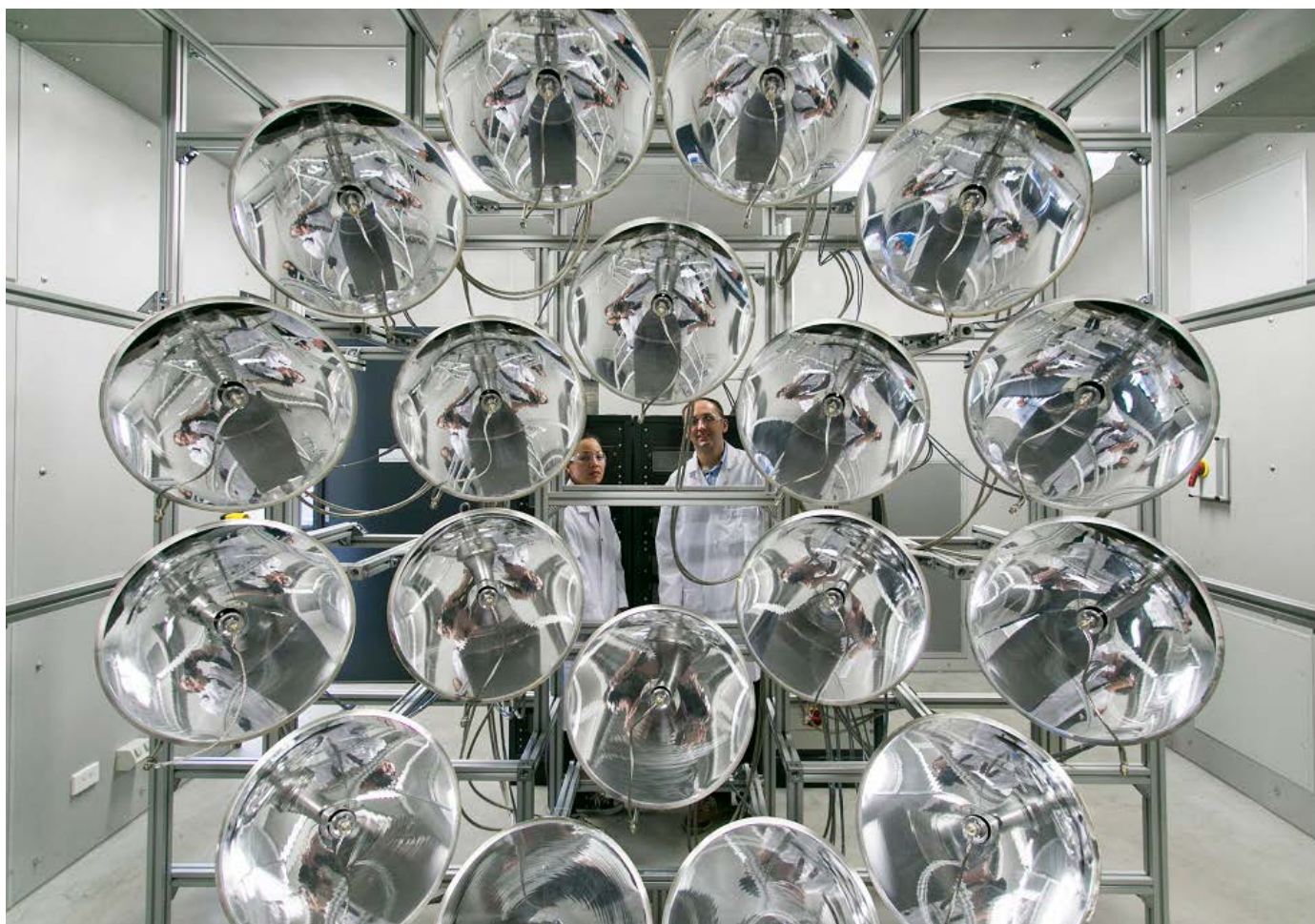
The ANU high-flux solar simulator, with Ms Lindsay Yue and Prof Wojciech Lipinski in the background. Photo credit: ACT Govt.
