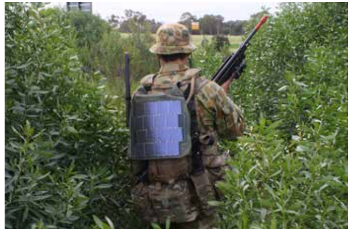
Photo: The wearable solar technology in use during trials (Department of Defence)
